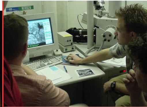
◀ The Center for Advanced Materials and Nanotechnology (CAMN) at Lehigh University offers students real-time remote access to their XL30 ESEM (environmental scanning electron microscope). To achieve acceptable scan rates requires the high level of performance that Internet2 provides.
