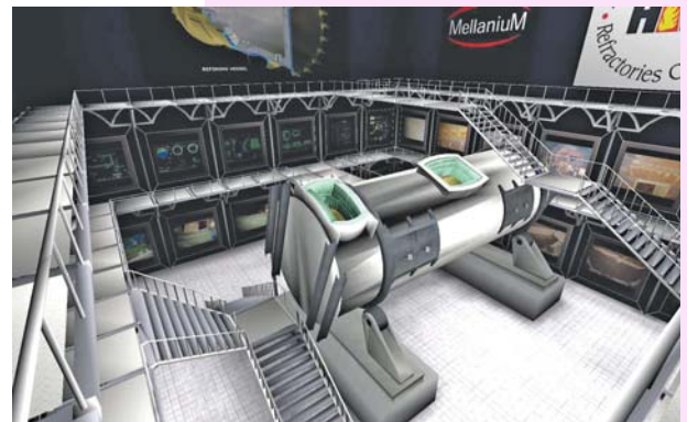
Figure 1. Web.alive rendering of a copper smelter. The 3D environment displays an accurate model of the anode vessel, showing the smelter and converter furnaces, including the design of the vessel's refractory lining.
