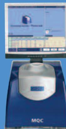
Reference values are compared against those calculated from the NMR calibration in Tables 1 and 2. The standard deviation over several measurements of the same sample is typically less than 0.1%. The standard error of estimate for these sets of samples provides an accuracy figure of 0.3% fat, although the accuracy can only be as good as the results of the reference technique against which it is being compared.
