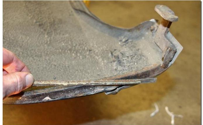
Original material was a thin gasket-like material glued to the lip of the fender skirt, not a rubber seal.
