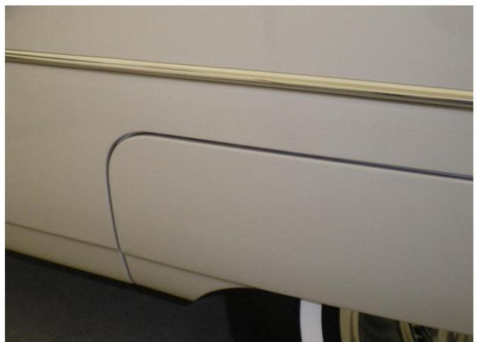
Fender Skirt with New Gasket Seal Now Fits Nice and Flush with the Body of Car
