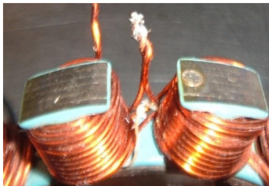
Figure 7 – Twisted wire connection
