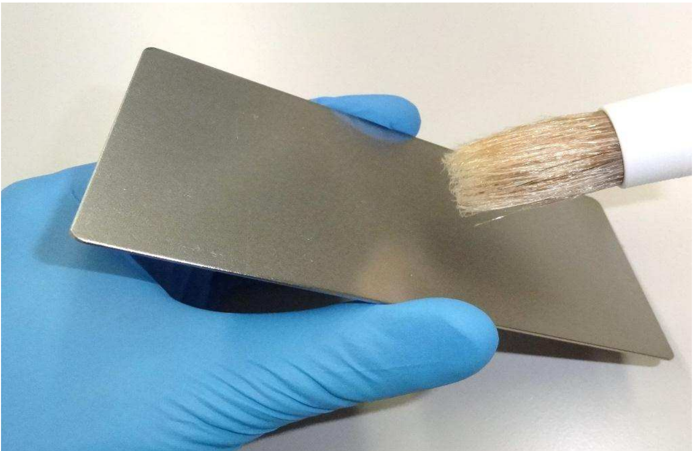
Picture 1: applying of ZF1 Liquid Protector with a brush
