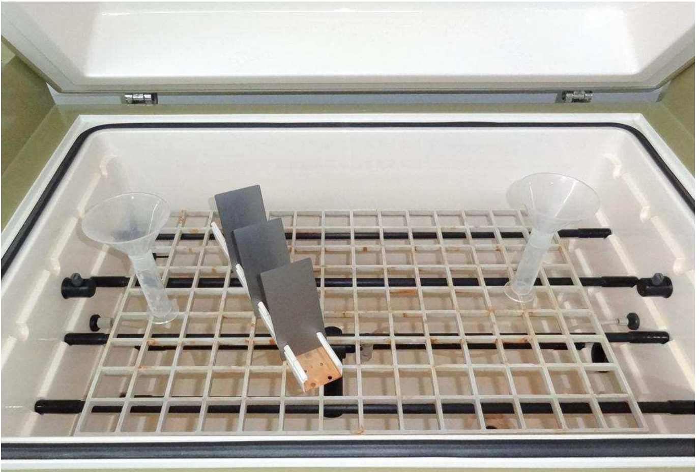
Picture 2: test setup in the salt spray chamber
