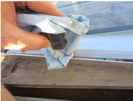
**Cleaning out the I-channel on the companion door. The screw driver works well to get the gunk out of the corners.**
