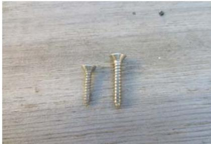
**The screws – The correct one to use is on the right – 1 ¼” #10 flat head stainless steel.**
