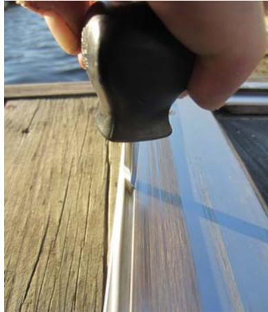
**A picture showing how I used the screw driver to put pressure on the slick strip after the adhesive backing was removed.**
