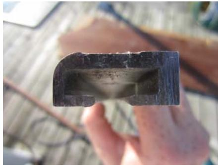
**A picture of the freshly removed "C-Channel" that attaches above the companion Doorway**
