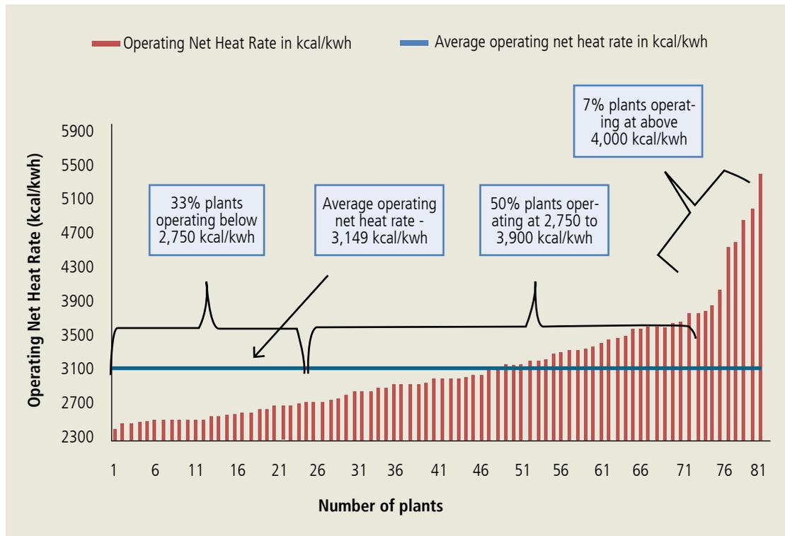
and have to meet the notified targets by March 2015. The minimum threshold of 30,000 MTOE of annual energy consumption is equivalent to a 20 MW power plant. This ensures coverage of all power plants commissioned before 2007 under this scheme. Energy reduction targets are given to each plant on the basis of its deviation of Operating Net Heat Rate (ONHR) from Design Net Heat Rate (DNHR).
