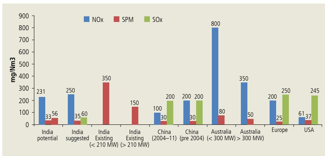
Post deployment of suggested combination of efficiency improvement and emission reduction, the emission limits of existing plants can be brought down to be at par with the norms of other developed countries and large emerging economies. For new plants, a similar comparison is done with the potentially achievable emission numbers vis-à-vis the present norms in other countries (Exhibit 29).
