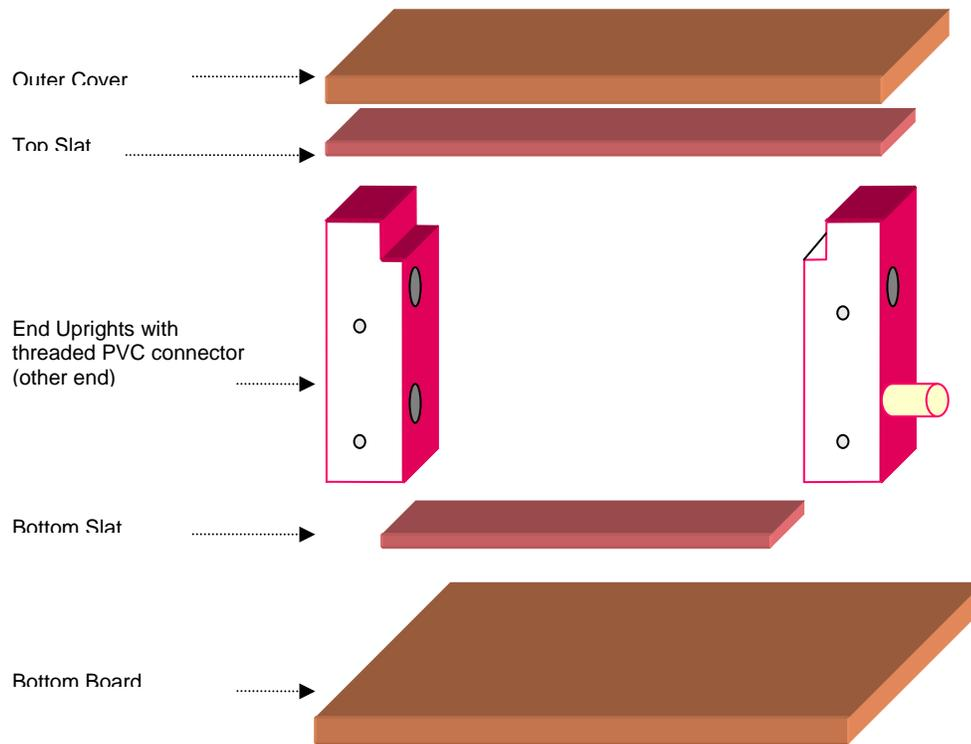
Figure 2. An exploded view of the observation hive.
