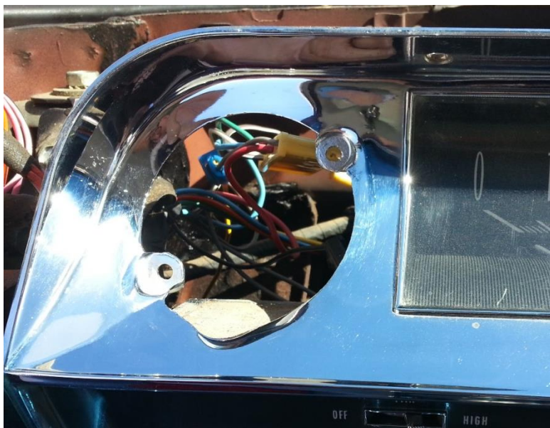
LEFT: Headlight switch bezel removed
