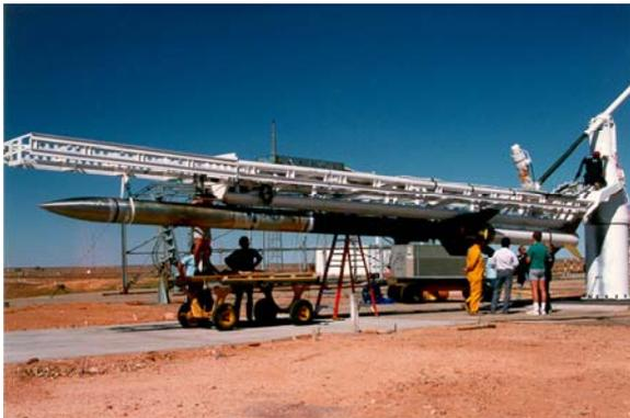
NASA sounding rocket trials have been conducted at Woomera on an occasional basis since 1961. The most recent series, involving solid fuel Terrier-boosted Black Brant rockets, were undertaken in 1987 and 1995 (total of 12 flights). The purpose of the flights was to carry out space-borne astrophysical research including observations of Supernova SN1987a which is best observed from the Southern Hemisphere.
