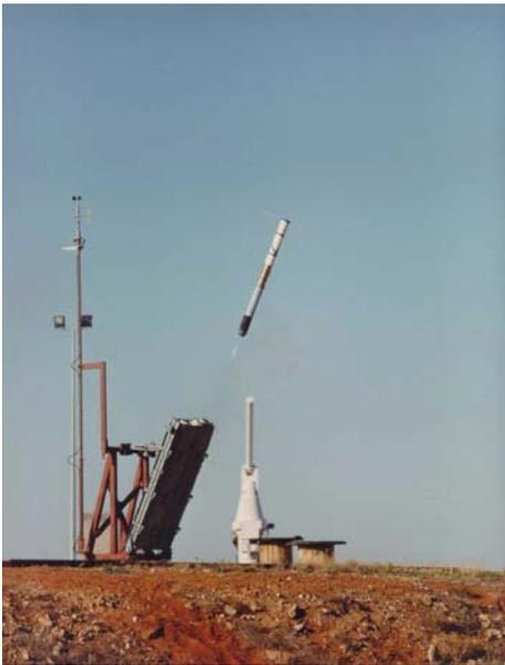
The Nulka hovering rocket is an Australian-developed, ship launched decoy used for protecting ships against missile attack. Powered by a solid fuel rocket motor, Nulka (Aboriginal word meaning ‘to be quick’) hovers away from its host ship, with its electronics package attracting the incoming missile by mimicking emissions from the target ship. Nulka is in service with the RAN, the US Navy and the Canadian navy.
