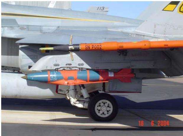
An F/A-18 aircraft operated by ARDU provided support in 2004 for a concept technology demonstration program involving the release of a GBU-38 Extended Range Joint Direct Attack Munition (JDAM). The trials were sponsored by Boeing / Hawker de Havilland, and required a large cleared range area to allow weapon release without a flight termination system.
