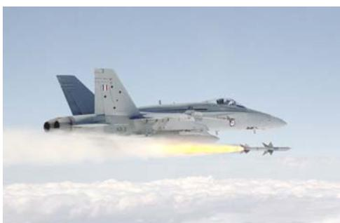
Two successful firings of the AIM-120 Advanced Medium Range Air-to-Air Missile (AMRAAM) were conducted at the WTR in April/May 2001 by the Aircraft Research and Development Unit (ARDU) of the Royal Australian Air Force (RAAF) with support from 77 Squadron. AMRAAM is a software-controlled, radar-guided missile that gives pilots the ability to 'launch and leave' and to track multiple targets during a single engagement.
