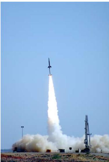
The HyShot program is led by the University of Queensland (UQ) and is aimed at testing advanced scramjet hypersonic propulsion. The program entails the launch of UQ scramjet engines on Terrier-Orion sounding rockets provided by DTI Associates. The rockets reach an apogee of over 300 km and a down-range distance of approximately 400 km. Activation of the scramjet engines occurs during re-entry at an altitude of approximately 35 km and a speed of around Mach 7-8.
