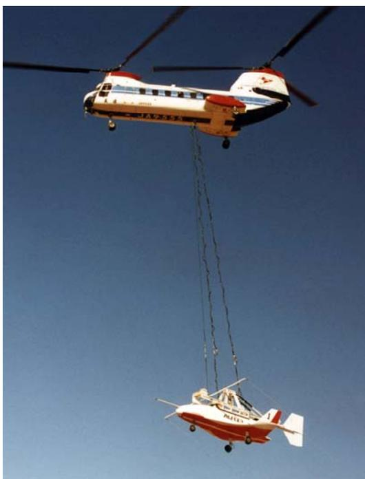
The Japanese Automatic Landing Flight Experiment (ALFLEX) entailed the testing at Woomera Airfield of a one third scale model of the HOPE spaceplane by the National Aerospace Laboratory (NAL) and the National Space Development Agency of Japan (NASDA). The objectives of the trials were to test the automatic landing technology to be used for HOPE. Selection of Woomera for the ALFLEX program followed a survey by NAL/NASDA of over 100 prospective sites in Japan and overseas.
