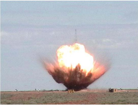
The WTR was selected by NASDA in conjunction with the Nissan Motor Company for the shock testing of propellant material from the Solid Rocket Boosters (SRBs) used on the Japanese H-IIA satellite launch vehicle. The purpose of the testing was to determine the explosive potential and fragmentation characteristics of the propellant, and in particular, to simulate the high speed impact of unburnt propellant as might occur in the event of a launch accident.
