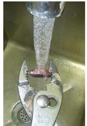
3. Measure the length of the thermowax. The overall length of the thermowax must be 23 mm or less during reassembly.
