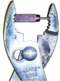
2. Place the thermowax under warm tap water (do not exceed 40° C or 104° F) and gently squeeze the pliers until the plunger is fully retracted. Be careful not to apply too much force or bend the thermowax plunger. Only 15 N (3.4 lb.) force is required to push the plunger in.
