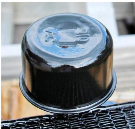
To the left and right the cap has been sprayed with 2 coats of Rustoleum Gloss Black engine paint. While it is not perfect, it is a huge improvement over the original condition of the cap!
