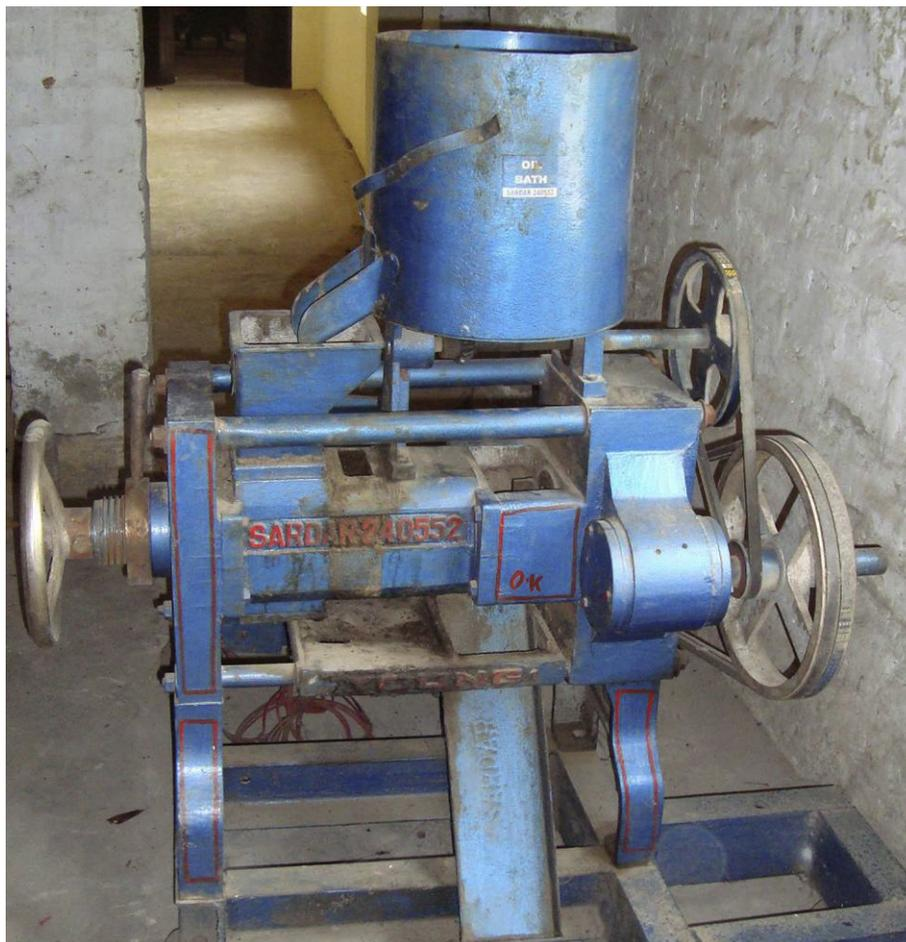
Fig. 1 – Screw press oil expeller.
