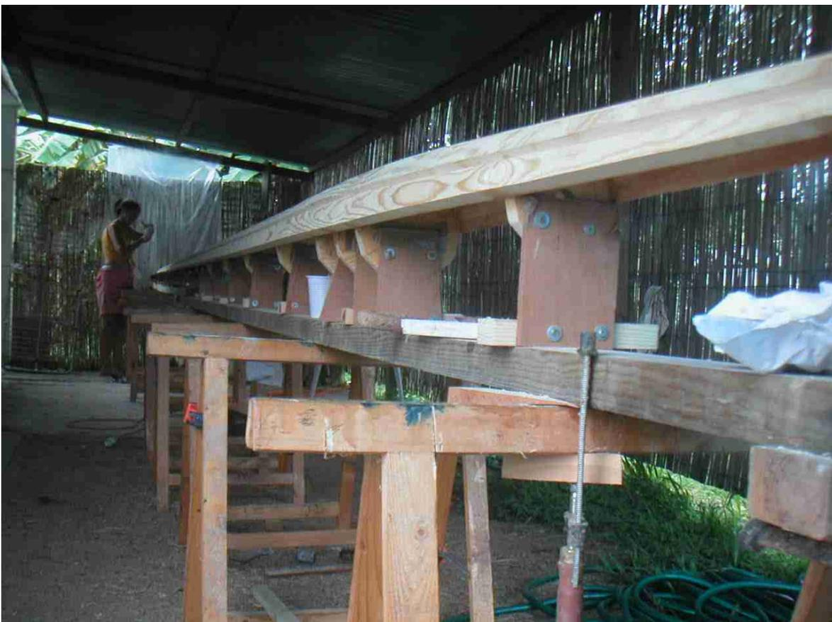
Now the “V” spaces between the staves are filled with a thick epoxy glue with no hurry :
