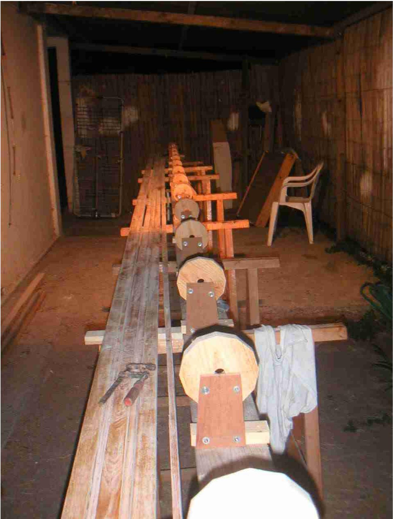
The first stave is glued on the bulkheads with the help of temporary screws :
