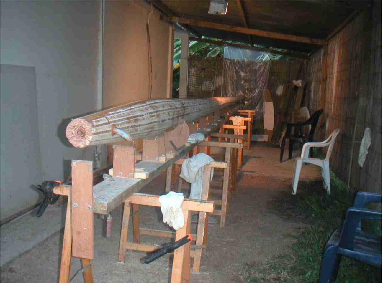
With its 12 faces, this mast is easy to round and after to have glassed the masts, unidirectional carbon cloth is added only on the bottom part above and below the deck level :
