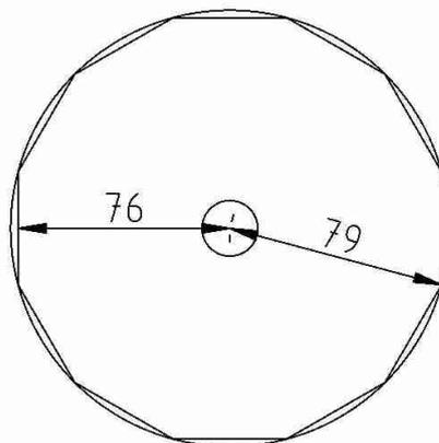
The mast shape is generated by the bulkheads which are fixed on a thick timber each 60cm . They are well aligned wit a thin line strongly tensioned between the foot and top of the mast :
