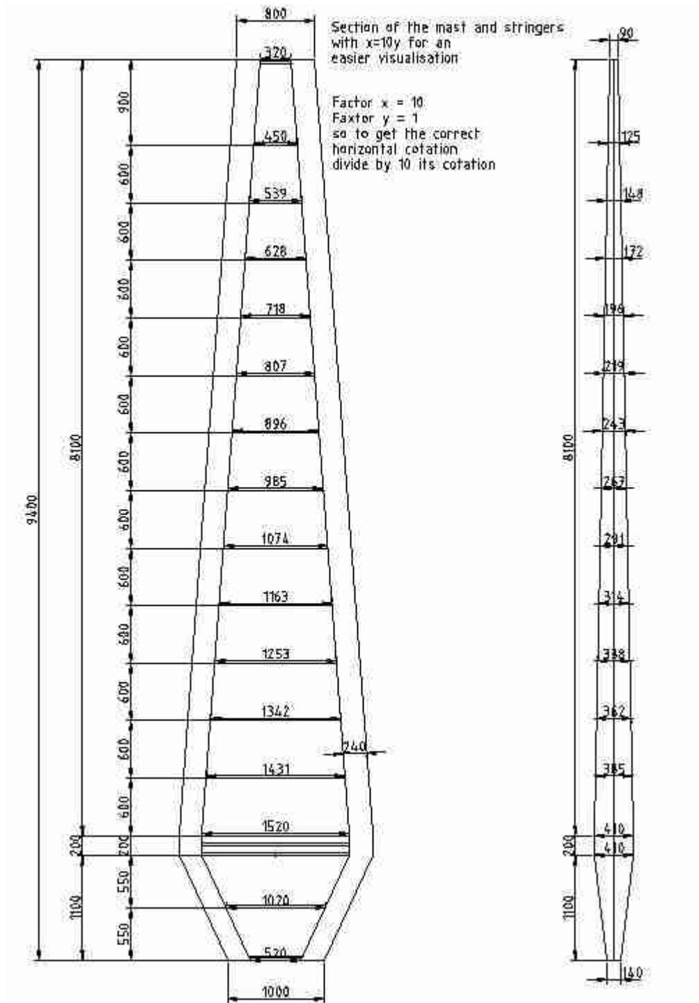
The first job is to cut the 12 staves in timbers of 24mm thickness and 10.50m minimum length. Why 10.50m? It's because with longer timbers than the total mast length it's possible to cut alternatively a stave from top and the next one from foot to avoid to waste wood.
