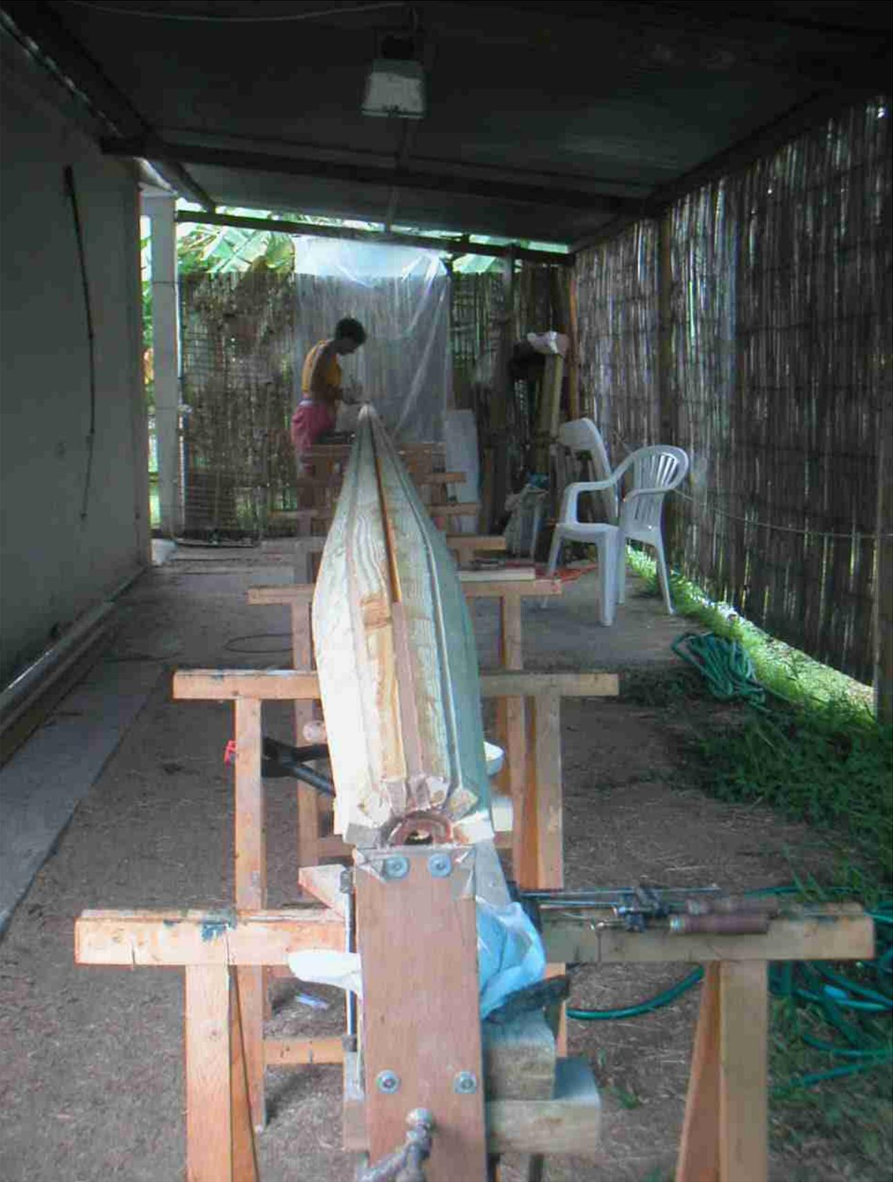
After to have glued so all the staves together, the half mast is disconnected from its support, turned and is well hold to keep it straight. Before to complete the mast a plastic tube is put through the center of each bulkhead :
