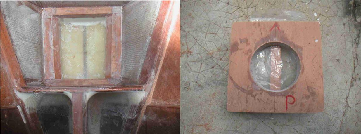
and a thick laminated plywood collar has been made moulded on the deck to follow exactly the shape of the deck. A thick rubber collar is put under the plywood collar in order to get a good sealing :
