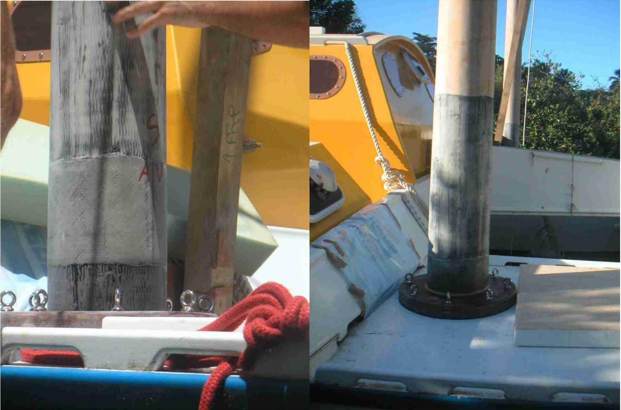
At the top, stainless eyes are bolted with epoxy to hold the blocks :
