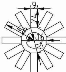
This mast is build as a bamboo with bulkheads of 12 faces all 0.6m to get a light and strong mast. For that I cut according my plan 18 discs with 12 faces in the same timber of 24mm thick.
