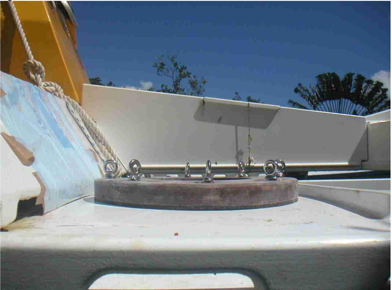
In order to adjust exactly the mast to the deck collar and keel, the mast is placed in the hull to be glued to the collar :
