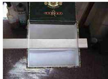
might want to use a few finishing nails as well. Be careful that you don't crack the lid when doing this. Use the finishing nails to close up the lid. I like to drill pilot holes so that everything goes in straight and easy. (Note: If you want to wire this baby for sound, see the note at the end of these instructions. Don't do this step yet!!)
