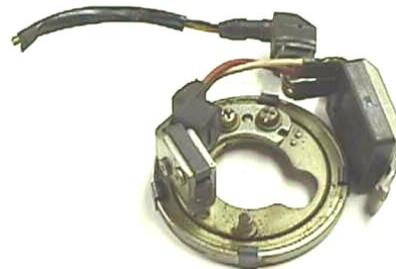
Grind, or cut and file the end of the pickups off as shown here. Make both pickups like the one on the right. If grinding, do not allow excessive vibration to damage the unit. Be sure to remove all the metal particles from the magnet areas.
