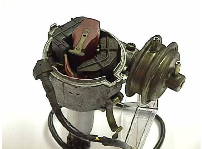
This is important so the rotor will line up properly with the cap to permit the spark to occur with the proper rotor location. Do not proceed until you are sure you understand what is needed here and make a permanent
