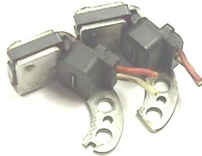
Test fit the pickups on the new plate.
