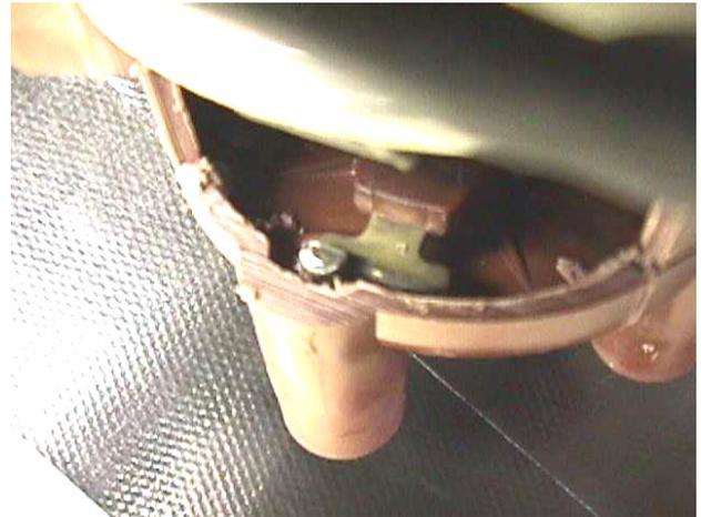
This may take a few tries to get where you want it. This step is very important, as the relationship of the rotor to the plug pickup post MUST be in line under the full range of advance. This is why the rotor tip is so wide. Now mark the plate position and or the pickup position so you can always remove and replace the plate to the exact position. A punch mark on the plate at one of the rectangular plate hold downs works for me.
