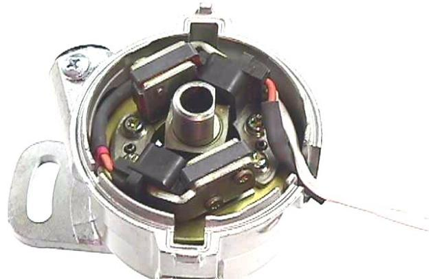
Both wires need to be bent to make the “U turn” inside the re-used grommet and through the slotted opening in the side of the distributor case. The final wiring bending and fitting into the grommet will be done later after the plate alignment is completed.
