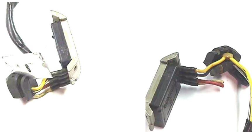
Now it is time to test fit the wired Pickups into the distributor. The first pickup is located approximately as shown with the wire looping around as shown. Use the 8-32 screws supplied with the kit. They will be tight the first time used, as the tolerance on the threaded holes is aircraft standards not automotive. Do not over torque, as the plate is aluminum. The screws are longer and thread the entire thickness of the plate
