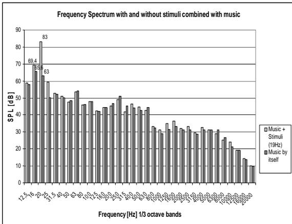
Figure 4. Level comparison between the test signals with and without the 19 Hz stimuli.
