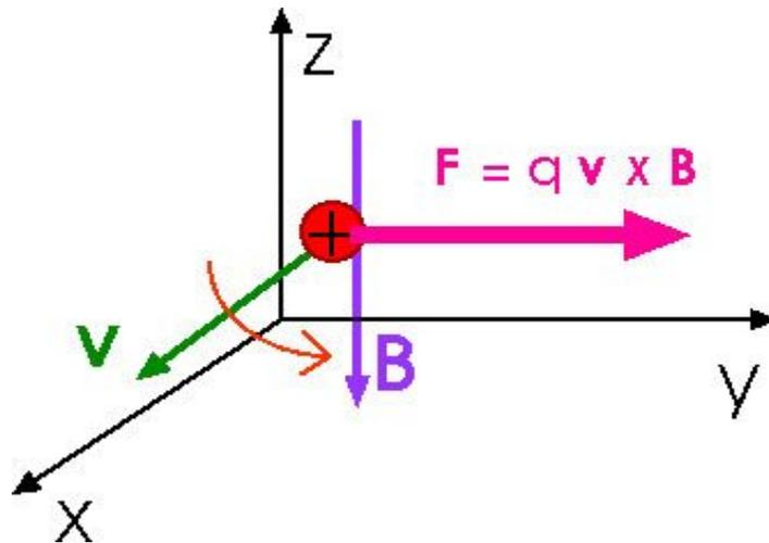
The vector  $\mathbf{v} \times \mathbf{B}$  points along the positive y-direction. For a proton,  $q$  is positive, so the Force vector  $\mathbf{F} = q \mathbf{v} \times \mathbf{B}$  also points along the positive y-direction. With a force on it in the positive y-direction, the proton will be moved from its initial path. The proton will move in a circle in a plane parallel to the xy-plane.
