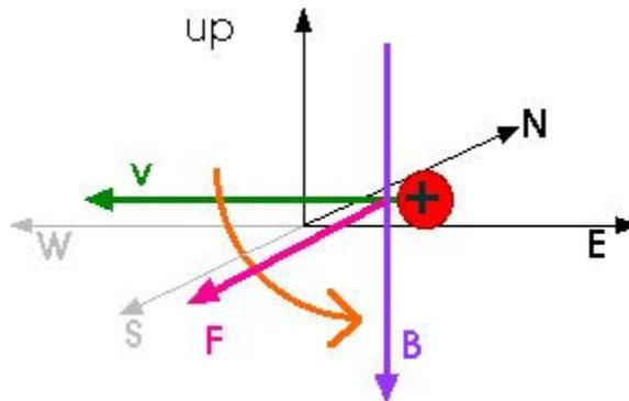
From the diagram we see that the force is directed to the **South**. Since  $\mathbf{v}$  and  $\mathbf{B}$  are perpendicular, the magnitude of the force is
