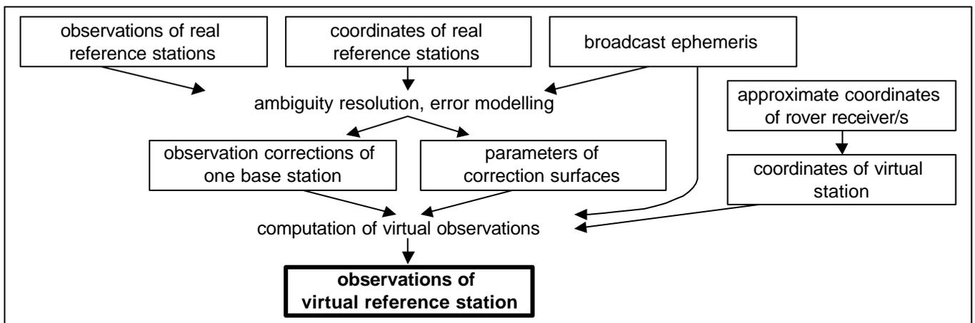
Fig. 2: Computation of carrier phase observations of a virtual reference station in a regional GPS-network.
