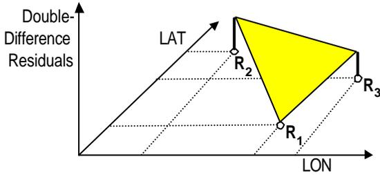
Fig. 3. Error modelling using bilinear surfaces are depicted best for double differenced observables. The actual algorithm is based on undifferenced observables.
