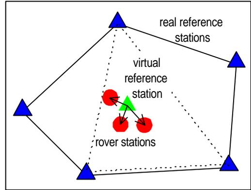
Fig. 1: Virtual GPS reference station in a regional network. The observations of the virtual station are computed from the observations of three or more real reference stations.
